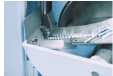
Rotary Hopper and Screw Orienting Wheel
