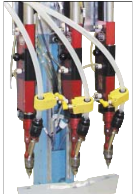
Three SD-2030 Driving Heads complete with feed system (not shown). Drives (3) #10 fasteners into a plastic dryer drum paddle at 35 in. lbs. (4Nm) torque.
