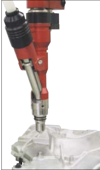
Model SD-2040 Driver with DC electric motor drives a M6 indented hex washer head screw with "thread locking patch" into a casting within a specific torque of 101 in. lbs. (11.5Nm).
