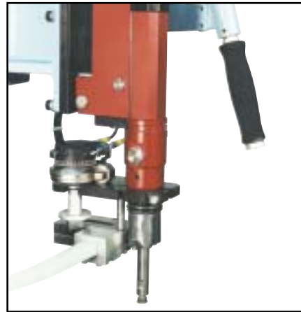
Model SD-2040 Nut Driver shown with vacuum tooling for a hex flange nut driving application.
