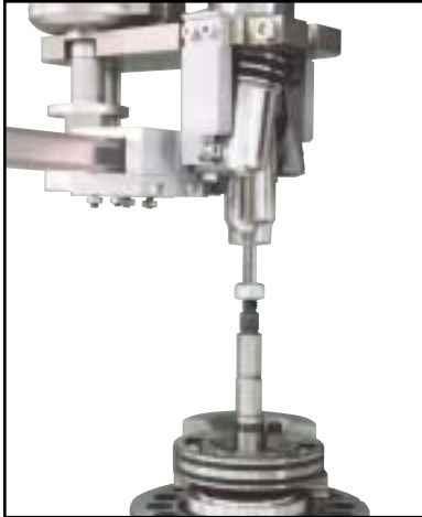
Model SD-2040 Nut Driver tooled with pneumatically powered centering pin and socket to drive a M8 hex nut onto a compressor assembly at 150 in. lbs. (17 Nm) torque.
