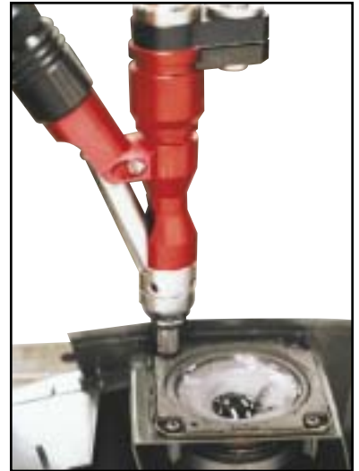
Model SD-2020 Driver with an electromagnetic particle clutch application. A #6 cross recess screw is driven into a speaker assembly within specific torque limits.
