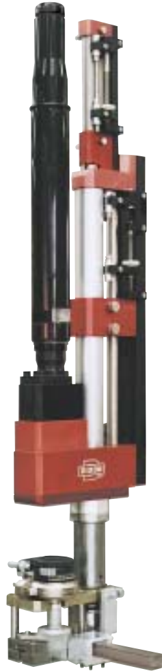
Model SD-2040 Nut Driver tooled with pneumatically powered centering pin and socket to drive a M8 hex nut onto a compressor assembly at 150 in. lbs. (17 Nm) torque.
