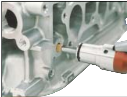
Model SD-2040 Driver tooled to drive a pipe plug "horizontally" into an engine block at 147 in. lbs. (16.7Nm) torque setting, \pm 3 Nm.
