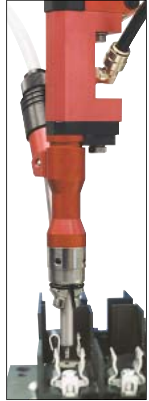
Model SD-2020 Driver shown with vacuum tooling to insert #2 Pozidrive screws between fuse clip barriers at 20 in. lbs. (2.25Nm) torque.
