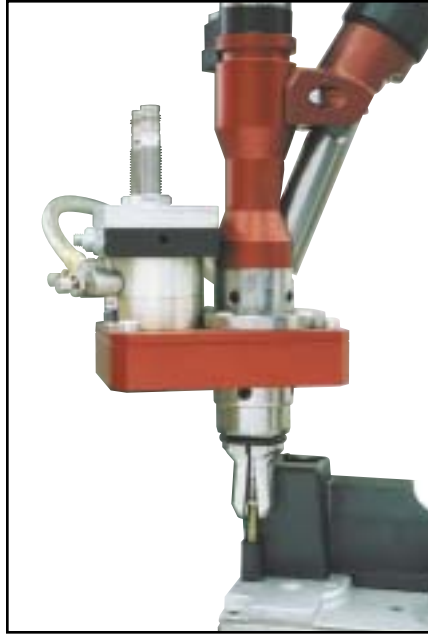
Model SD-2020 Driver equipped with a rotating jaw attachment in order to reposition the jaws to clear restrictions in a workpiece. The jaws can be rotated at various locations on the workpiece as required.
