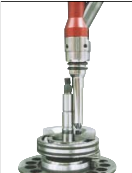
Model 2040 Driver with DC electric motor and "extended jaw" tooling. Two M4 Torx fillister head screws with captive lock washers. The fasteners are driven into a compressor assembly at two separate stations. Our engineers sometimes refer to this extended jaw as a "beak jaw".
